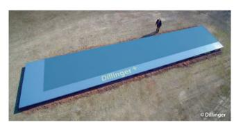
Rolled from a 600 mm slab and featuring the imposing dimensions of  $70 \times 4,200 \times 22,500$  mm - the world's largest ever continuous cast and thermomechanically rolled plate. The outline on the plate emphasises Dillinger's dimensional lead over the largest product available from any competing steelmaker.
